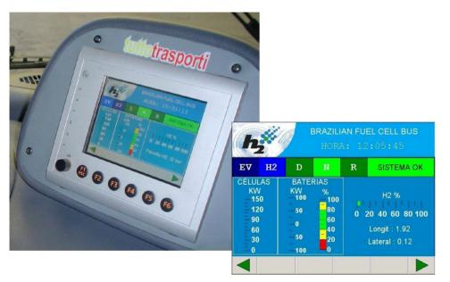
The great amount of information that flows through the vehicle electronic control systems made the performance data collection possible without the need to use complex measuring
