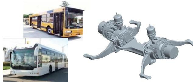
**Electric low-floor axles with ELFA induction ASM-Motors offer wide aisles at very low floor heights**
