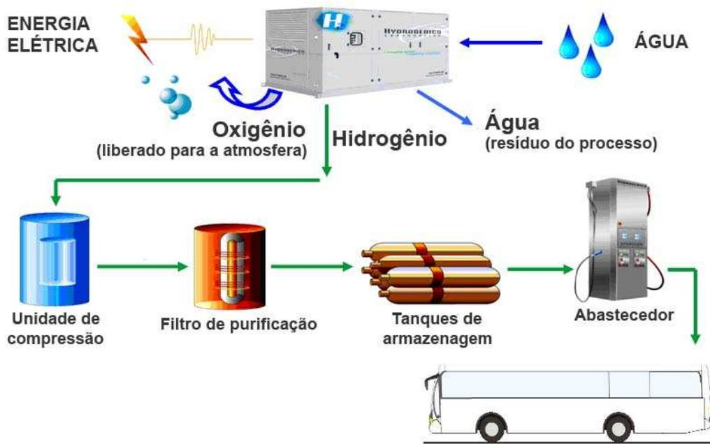
Incoming water will be purified via a reverse osmosis system. 50% of the water will be of high enough quality to be used in the hydrogen and oxygen production process. The remaining water, with high mineral content, is not suitable for drinking, but it will be used to water the gardens and clean the buses.
